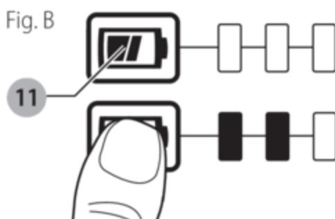
**NOTE:** The fuel gauge is only an indication of the charge left on the battery pack. It does not indicate tool functionality and is subject to variation based on product components, temperature and end-user application.
