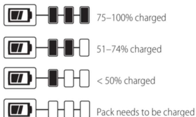
To actuate the fuel gauge, press and hold the fuel gauge button 11. A combination of the three green LED lights will illuminate designating the level of charge left. When the level of charge in the battery is below the usable limit, the fuel gauge will not illuminate and the battery will need to be recharged.
